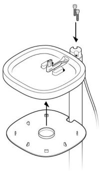
5. Plug the power cord back into the speaker and place on the top mount, pulling any extra cable down from the top. Tighten the screws and attach the top cap with the notch facing toward the speaker.
