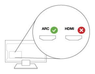
2. Connect the HDMI cable to the TV's HDMI ARC port.
