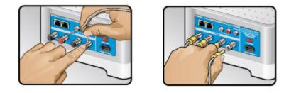
If your speakers have banana connectors, you can insert the plugs directly into the banana jacks on the back of the Connect:Amp instead.
