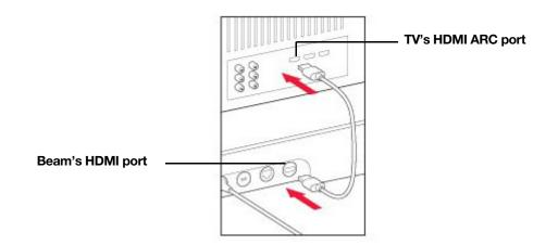
Note: If you can't find the word "ARC" on the label, it isn't the correct port. See <u>If your TV doesn't have an</u> <u>HDMI ARC port</u>.
